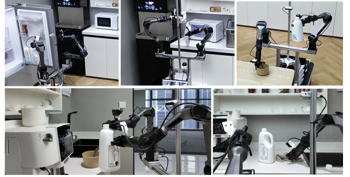
Fig. 8: A long-horizon episode of our robot in a kitchen. Sub-tasks such as opening the fridge door, opening then placing items into a microwave, fetching and pouring milk, and wiping a bench.
